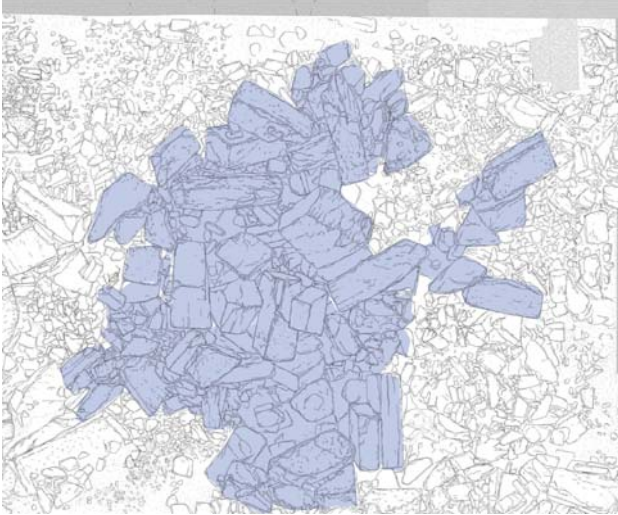
Figure 12. The stoneblocks of the NE corner of the tower after their collapse.
