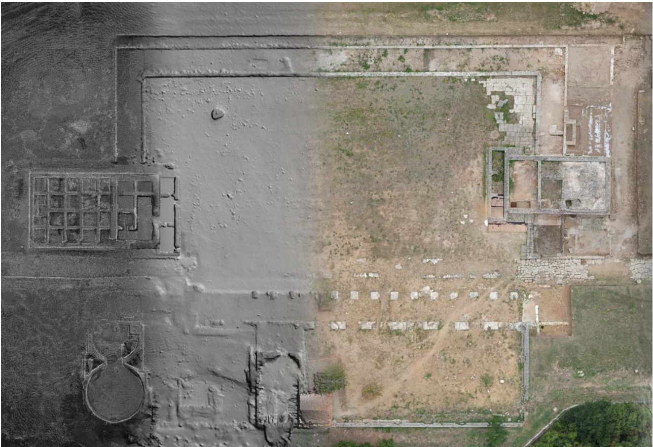
fig. 1 from point clouds to DEM, to ortho-image of Grumentum forum
