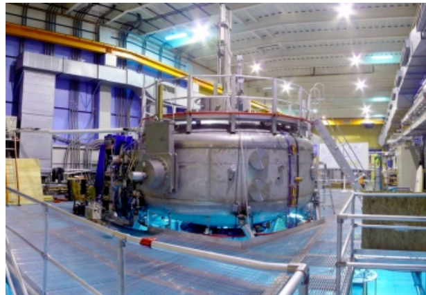
The Levitated Dipole Experiment (LDX) reactor is housed inside a 16-foot-diameter steel structure in a building on the MIT campus that also houses MIT's other fusion reactor, a tokamak called Alcator C-mod. Photo courtesy of the LDX team
