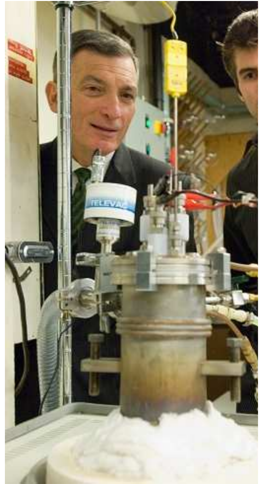
Professor Donald Sadoway and graduate student Bradwell observe one of their small test batteries in the lab. The battery itself is inside the heavy-duty stainless steel cylinder at center, which heats it to 700 degrees Fahrenheit while the wires at top charge up the battery and test its performance. Photo: Patrick Gillooly
