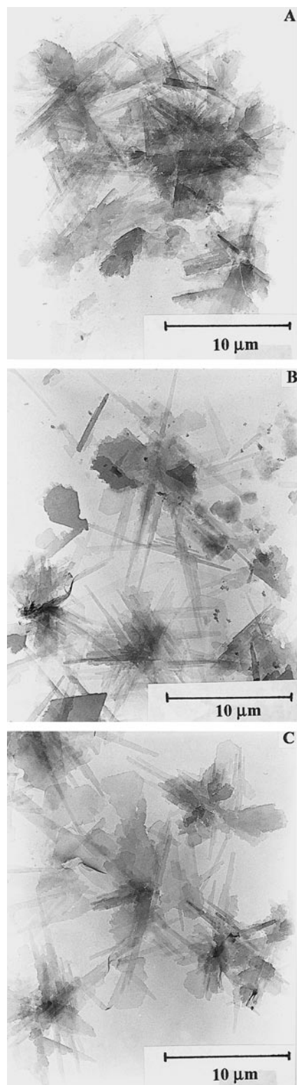
FIGURE 6. Transmission electron images of illite particles created by hydrothermal treatment of the gel for (A) 24 h, (B) 7 d, and (C) 28 d.
