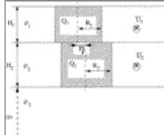
FIG. 1. Configuration used in this study. We consider a 2-layer system above an infinitely deep bottom layer. The vortex is composed of two PV patches (one in each layer) with radii R_1 and R_2 and strengths Q_1 and Q_2 in layers 1 and 2, respectively. Here, \mathbf{D} represents the separation between the PV patch centers. A background current (\bar{U}_1, \bar{U}_2) is also taken into account
