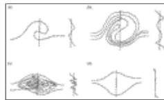
Fig. 1. Schematic of a turbulence entraining a patch of heavier water into the upper layer (a) and molecular diffusion of salt and heat occurring. Turbulence continues to strain the patch while its salinity and temperature anomaly decreases (b). If the turbulence stops, the patch, if not completely diffused away, will sink during the restratification process (c).
