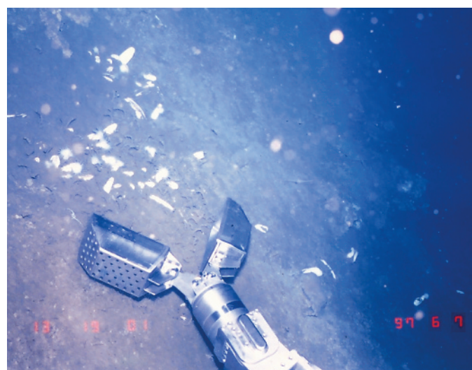
Fig. 2. Photograph of the sampling site of Calyptogena phaseoliformis with the manipulator of the submersible Shinkai 6500 of the Japan Marine Science and Technology Center. The size of the scoop shovels at the clamp of the manipulator is 20.4 cm in length, 12.2 cm in width, and 9.0 cm in height.
