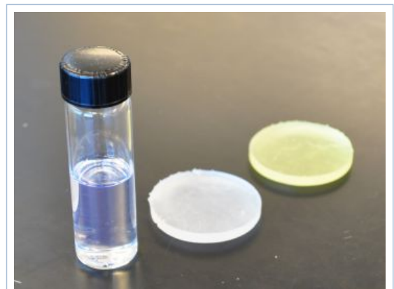
From left, 3D printing liquid, 3D-printed piece from liquid resin and liquid resin piece treated with ultraviolet light.
