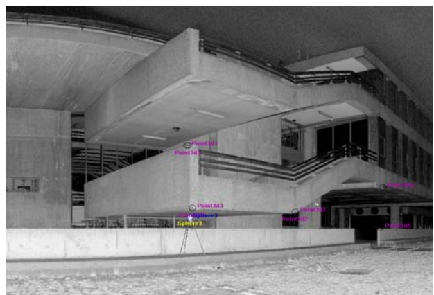
Figure 9. Registration using spherical targets in FARO Scene
