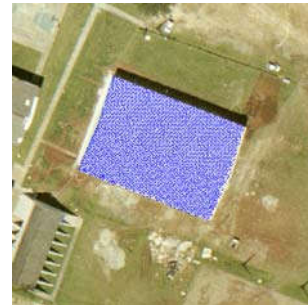
Figure 3: Interpolated LIDAR points on the roof
