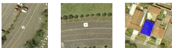
Figure 4: Type of pre-signalized control points and a typical centroid point determined
