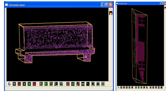
Figure 4. Generating extrusion outline (Left: an extrusion with one façade face; right: an extrusion with two façade faces)
