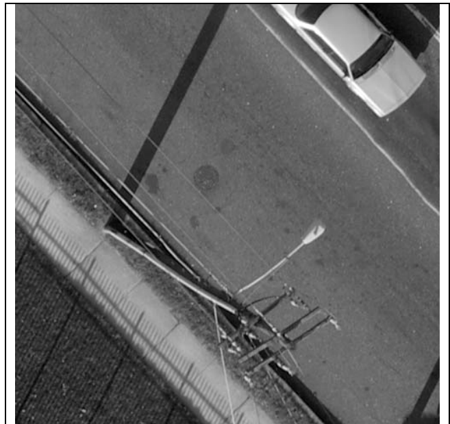
Fig. 3: light pole and power line with 2.2cm GSD
