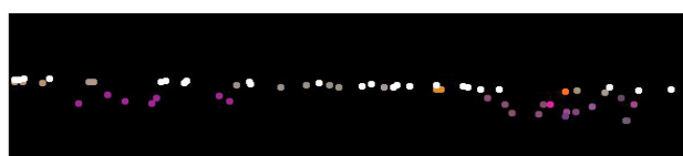
Figure 2. The cross-section of ALS data reveals how some echoes are shifted downwards from the asphalt level when hitting the white road markings.
