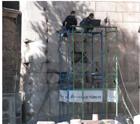
Figure 5 – A scan acquisition from the trestle of a portion of one of the Latin epigraphs
