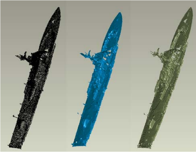
Figure 4. Results of Point Phase, Polygon Phase and Shape Phase of the deck
