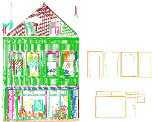
Figure 6. An example showing an extracted window is smaller than reality, as a result of obstacles on this window
