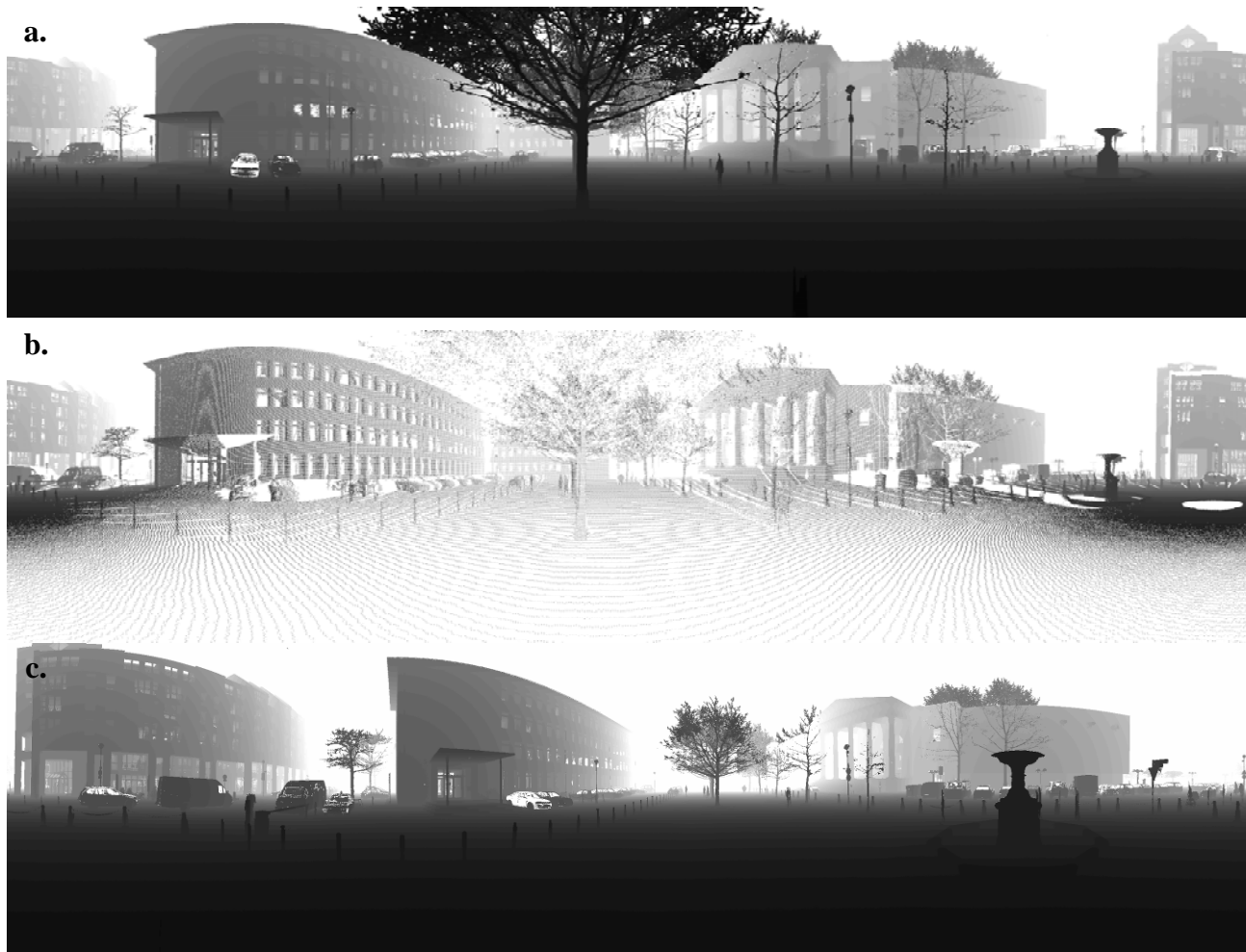
Figure 5. a. Reference scan. b. Analyzed scan transformed into the reference frame. c. Analyzed scan in its original local frame (not transformed).
