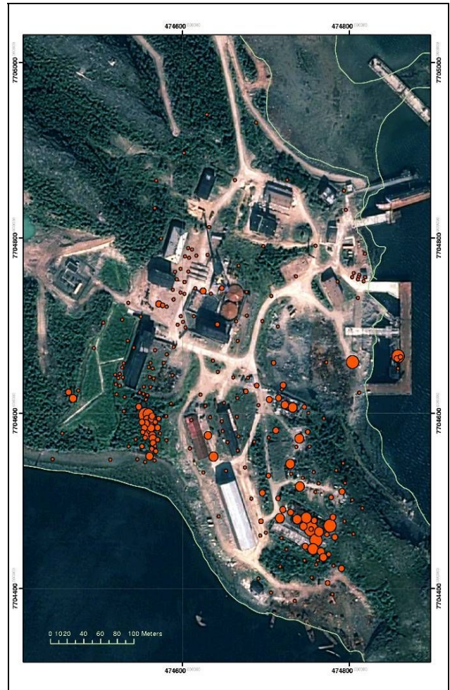
Figure 11. Sampling points for measurements of radionuclide concentrations (Cs-137, Sr-90). Values shown for Sr-90.
