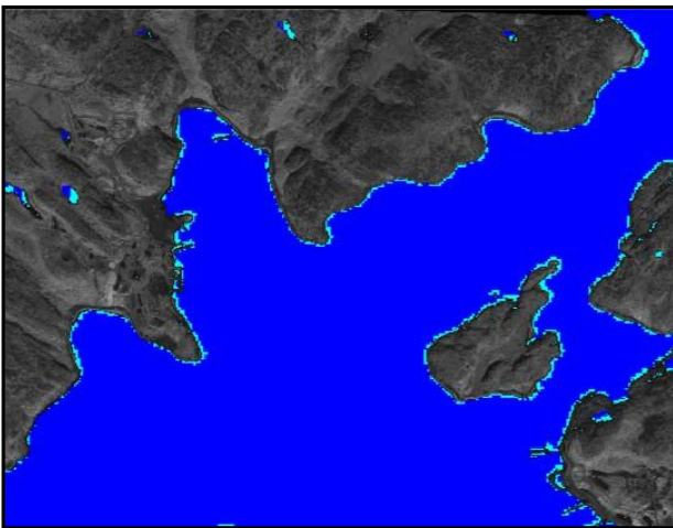
Figure 6. Comparison between water-mask derived from orthorectified Landsat-7 ETM+ near infrared band 4 and QuickBird sub-scene after georeference adjustment.
