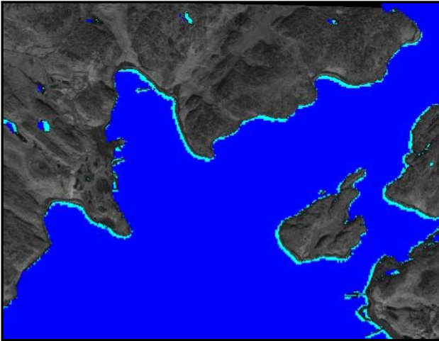
Figure 5. Comparison between water-mask derived from orthorectified Landsat-7 ETM+ near infrared band 4 and original system corrected QuickBird sub-scene.
