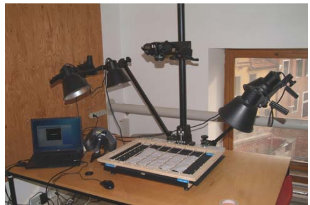
Figure 5: The acquiring system: handyscan, notebook, digital camera, 3D grid and light device.
