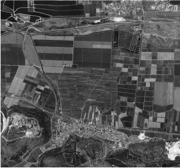
Figure 5: Rectified ortho-image after the parameter estimation
