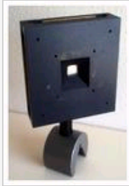
Figure 4: 128 \times 128 electrically addressed liquid crystal SLM constructed by LETI (France) in 1975.
