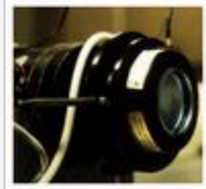
Figure 5: Optically addressed liquid crystal light valve manufactured by Hughes Corp in 1978. The photo shows the light valve coupled to a CRT.
