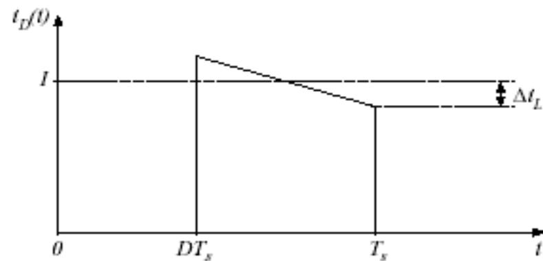
Minimum diode current is  $(I - \Delta i_L)$
