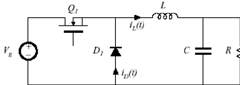
Minimum diode current is  $(I - \Delta i_L)$
