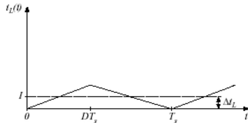
Minimum diode current is  $(I - \Delta i_L)$
