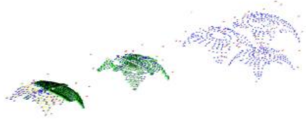
Figure 8. The final result: a 3D model of all vaults in one reference coordinate system after importing to AutoCAD. The measured points are displayed in blue colour, outlines of the bricks are in green colour and red points show control points used for the final 3D model.
