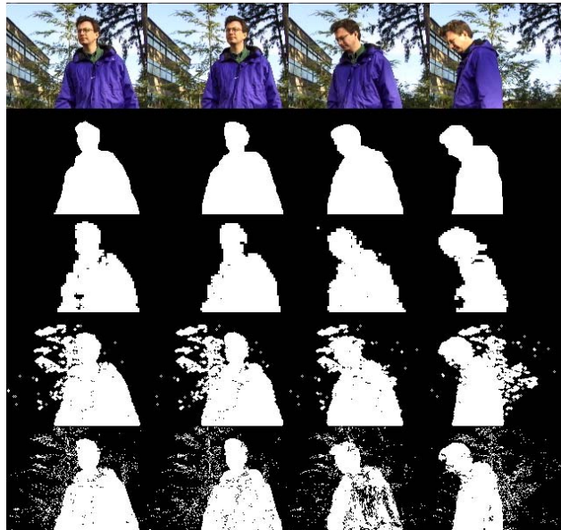
Fig. 2. Comparisons results on waving trees sequence. the top row are the original 247 th , 249 th , 254 th and 256 th frames, the second row are the ground truth frames, and the third row results are obtained by the proposed method. The fourth and fifth rows are the results obtained by MOG and KDE, respectively. Note that morphological operators were not used in the results.
