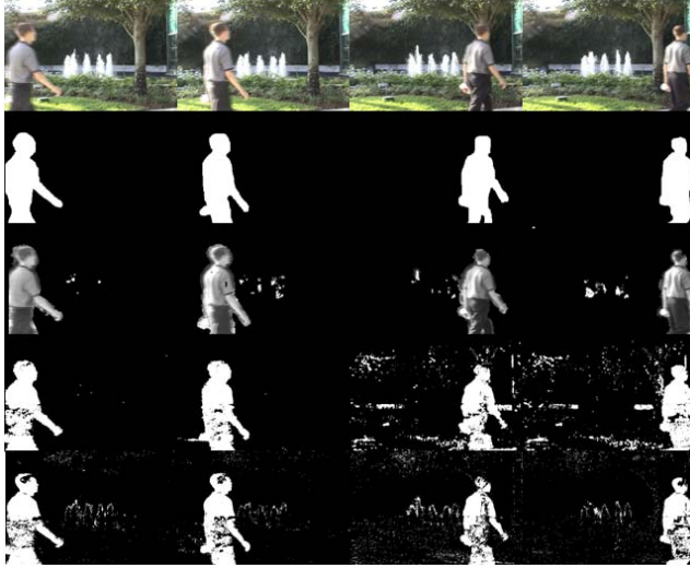
Fig. 3. Comparisons results on fountain sequence. the top row are the original 594 th , 598 th , 610 th and 616 th frames, the second row are the ground truth frames, and the third row results are obtained by the proposed method. The fourth and fifth rows are the results obtained by MOG and KDE, respectively. Note that morphological operators were not used in the results.
