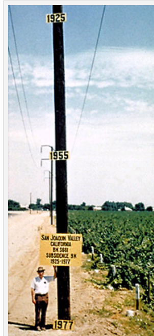
Pole showing the approximate altitude of the land surface in 1925, 1955 and 1977 at a site in the San Joaquin Valley southwest of Mendota, Calif., where researchers identified the approximate location of maximum subsidence in the United States. Photo Courtesy USGS.
