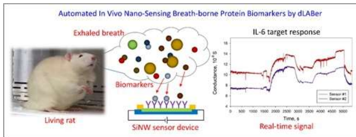
Detection of Living Animal's Exhaled Breath Biomarker (dLABer) 系统示意图
