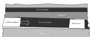
Fig. 1. Vertical section of location relationship between No. 3 coal seam and No. 4 coal seam.
