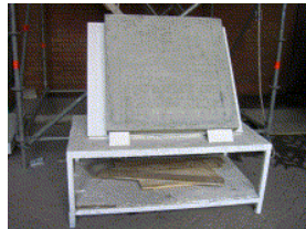
Fig. 4. A support for holding concrete blocks.
