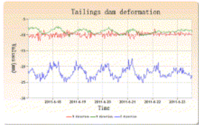
Fig. 4. The TDMPAS real time 3D deformation monitoring data graphically.
