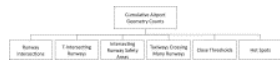
Fig. 3. Factors related to cumulative airport geometry , to be used in factor hierarchies.
