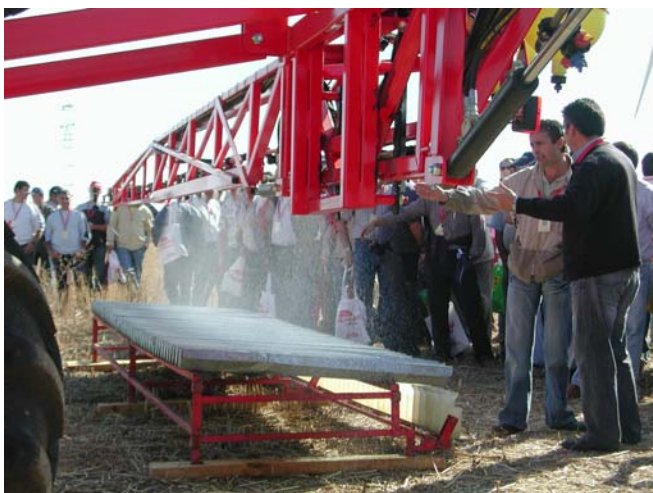
Training farmers and technical operators on spray distribution with low-drift nozzles in North Spain.
