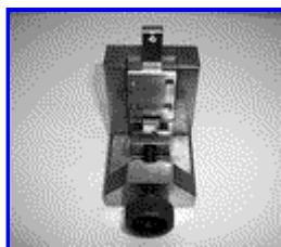
Figure 1. Overall view of the shearing rod used for performing shear bond strength tests
