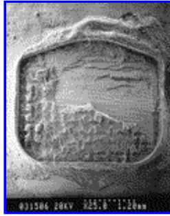
FIGURE 1. SEM (25x) shows the enamel surface after debonding in metal bracket—System 1+ group. ARI score = 1. Enamel fracture is noted
