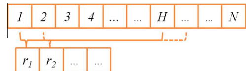
Fig. 3. Schematic of rolling horizon decision making in reservoir operation ( H is assumed equal to N in this study).
