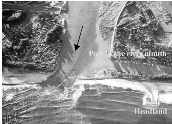
Photo 3 Flushing of the sand bar (Nov.7,2002)
