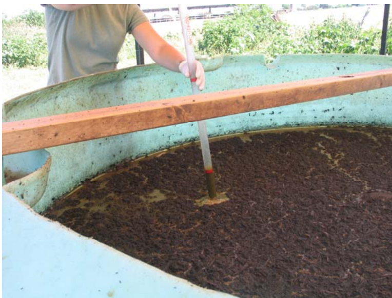
Figure 3. Tank sampling during the L4DB ® Microbial Treatment System demonstration
