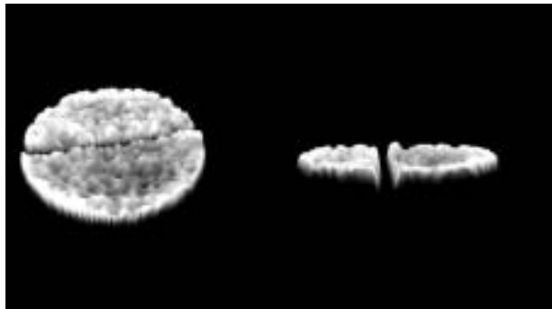
图 7 含裂缝试样不同视角方向的三维 CT 图像 Fig.7 3D CT image in different viewing directions of the specimen with crack
