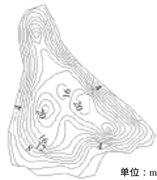
图 3 滑面埋深等值线 Fig.3 Contours of buried depths of sliding surfaces
