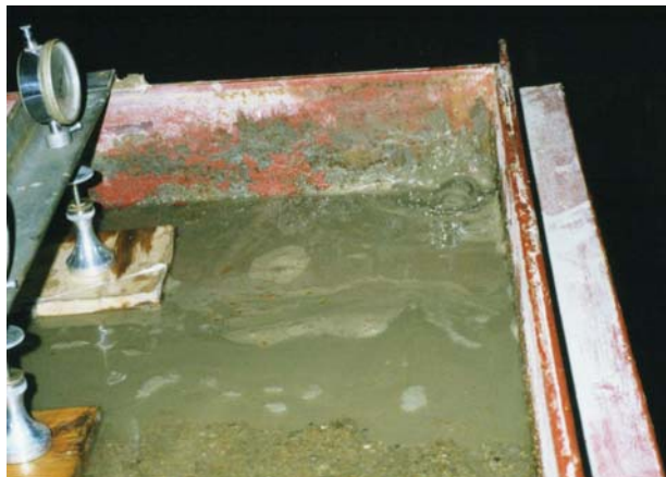
图 1 基坑突水破坏(喷出高度达 5 mm 的浓浓泥浆水) Fig.1 Failure of water gushing in pit(dense mud fluid with a gushing height of 5 mm)
