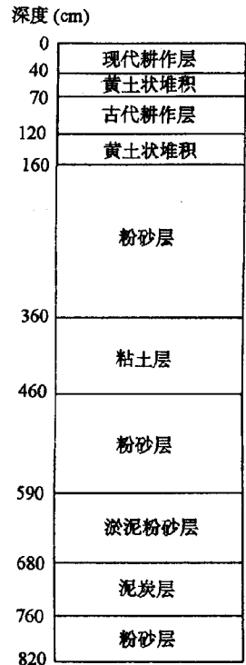
图1 北京房山东甘池东剖面岩性图 Fig. 1 Lithologic section diagram in east profile, Dongganchi, Beijing
