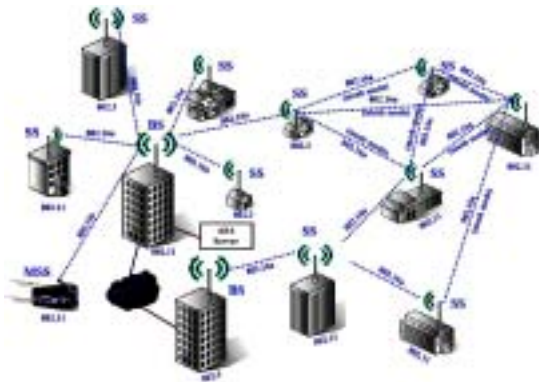
Fig.1 The architecture of WiMAX network
