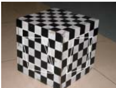
(a) Image of calibration object and trapezia (a) 标定块图像和梯形
