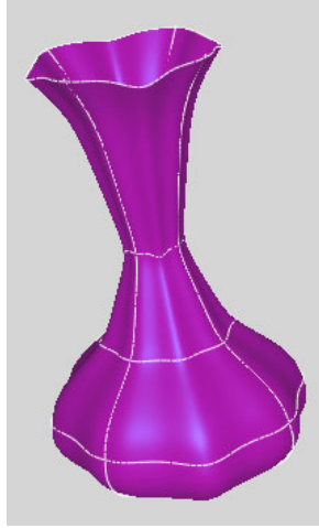
(b) The interpolation subdivision surface, where the highlight curves are the interpolated curves (b) 细分插值曲面,其中亮线为被插值曲线
