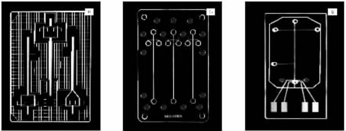
图 2 作者所在课题组研制的玻璃芯片(a)、PMMA 芯片(b)和 PDMS 芯片(c) Fig.2 Glass microfluidic chip (a), PMMA microfluidic chip (b) and PDMS microfluidic chip (c) developed in the authors' lab
