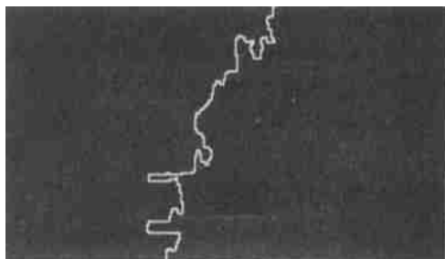
图 7 冬小麦地中阈值分割算法检测出的行走路径 Fig. 7 Walking path detected by threshold segmentation in the winter wheat field
