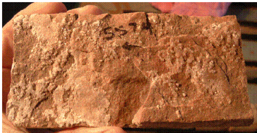
(a) A natural fracture face that is partially covered with crystalline dolomite
