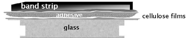
Figure 1. Schematic representation of the specimen preparation.
