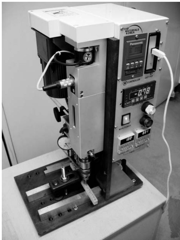
Figure 2. Photo image of torque tester (Biomaterials Korea Inc, Seoul, Korea).
