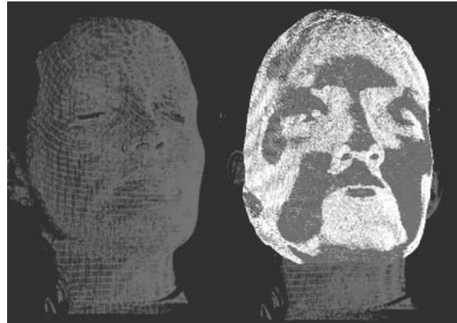
FIGURE 5. Facial point cloud of a proband (left) matched with the point cloud of his facial plaster cast (right).
